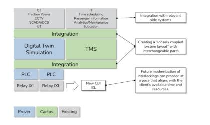
A key feature of this architecture is the integration platform, which acts as a layered structure separating different components. This modular approach ensures that individual elements such as the digital twin, TMS, or PLCs can be upgraded or replaced independently without affecting the entire system.
